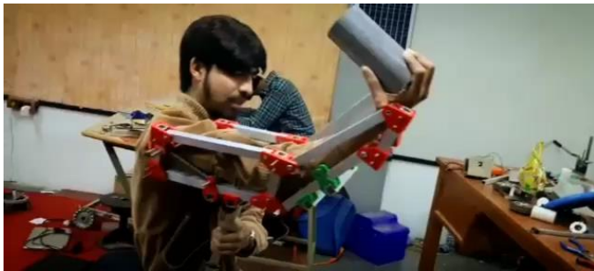
Arm Model With 90° Extension with emg sensors
