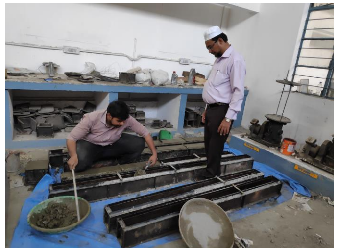
Preparation of Beams for carrying out the testing
