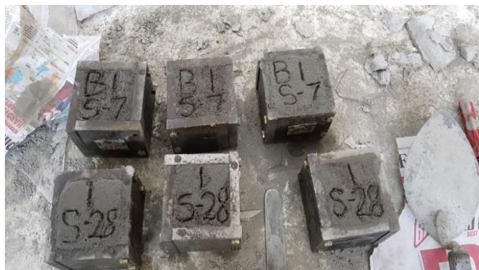
Samples prepared to determine the compressive strength of ordinary Portland cement after mixing of Nano- particles
