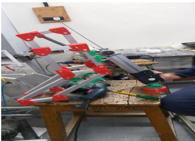
Structural Arm Model with Linear Actuator
