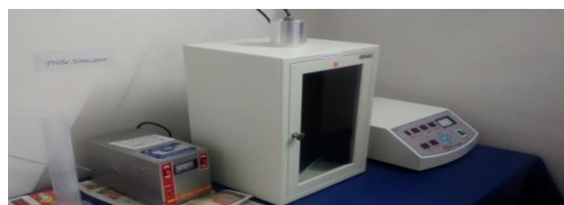
Preparation of CuO Nano fluid using Ultrasonic probe sonicator
