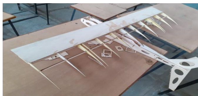
Model in making using Balsa wood with Laser cutting
